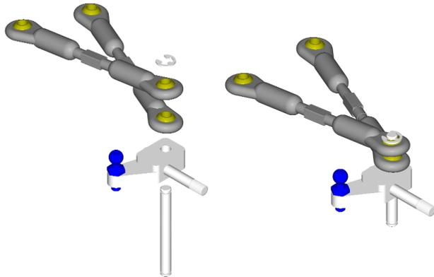
Locating the kingpins (x2), and the previously assembled front links and steering blocks, along with 1/8" E-clips, assemble as follows; Install the kingpin into the steering block to about the middle of the kingpin. Next, slid on the longer link (front) first followed by the shorter link (rear). Install the E-clip onto the top of the the king pin. Now slide the steering block to the top of the kingpin, taking up the slack at the top of the kingpin.
