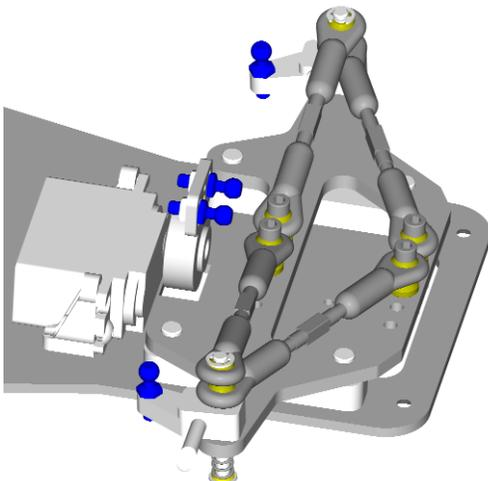
After carefully marking the center of the servo mounting holes, place the assembled servo back on the chassis to make sure the marked holes appear where they should be.
