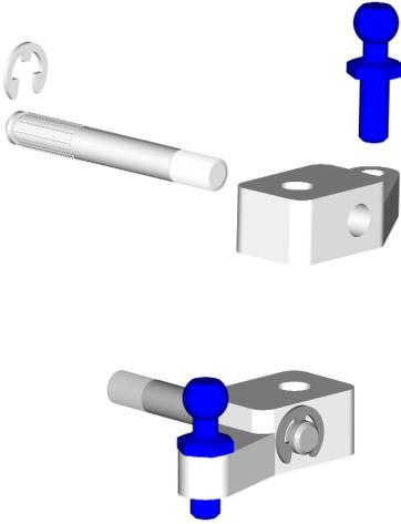
Attach the E-clip into the groove in the front axles (x2), being careful to protect your eyes in the process. E-clips that have not seated properly can become unpredictable flying objects and can do serious damage to sensitive areas on the body (like eyes).
