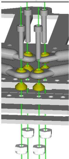
Using the 4-40 x 5/8" socket head cap screws (x4), brass cone washers (x4) and large 4-40 lock-nuts (x4), attach the links to the lower arm. Slide the screws through the captured ball ends then through the cone washers, then thread them into the holes closest to the center of the chassis. Keeping a hex driver in the screw, use a nut driver to install the 4-40 nuts from below the chassis. The screws should be held snug to the carbon lower arm when tightening the nuts.
