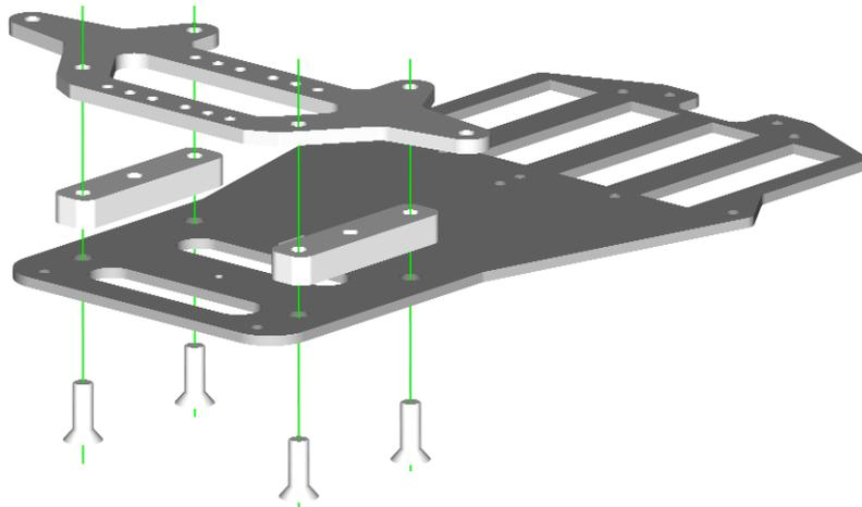
Using the provided stainless steel 8-32 x 1/2" cross point (Phillips) screws (x4), attach the lower front suspension arm (be sure the pockets for the pivots are facing down). The screws will thread into the holes shown. Be sure to keep the plate as even as possible, tightening opposite screws a little at a time equally. This will ensure that attaching these two plates together will not introduce any tweak into the chassis. Do not over tighten.
